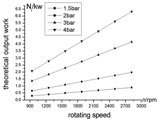
Figure 14. Theoretical expander output work.
