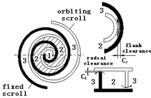
Figure 3. Radial and flank leakage model.
