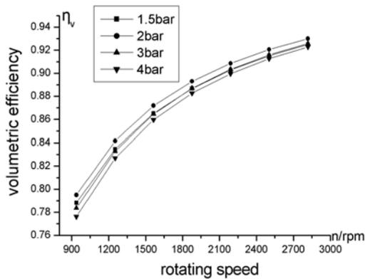
Figure 10. Volumetric efficiency.
