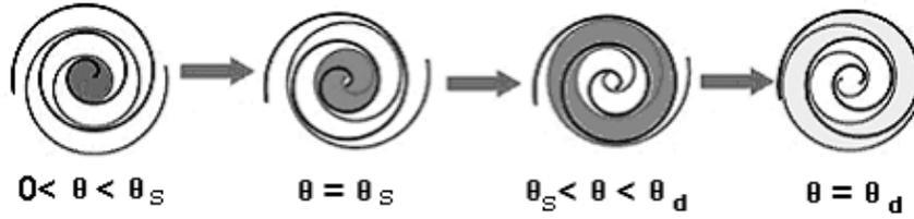
Figure 2. Working principle of the scrolls.
