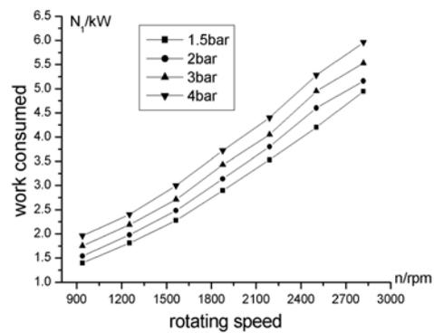
Figure 12. Electric power consumed by compressor.
