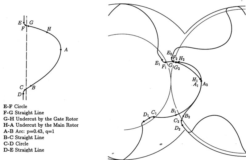
**Fig. 4 'N' Screw Rotor Profile**
