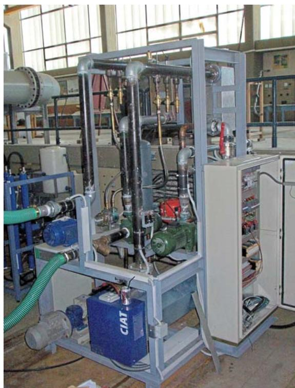
Fig. 2. The Rankine engine.
