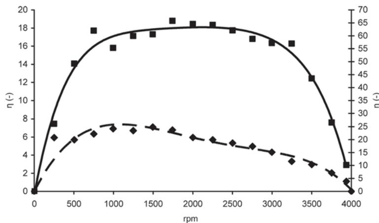
Fig. 8. Variation of the expander efficiency (continuous line, right axis) and overall system efficiency (dashed line, left axis) as a function of the rotation speed.
