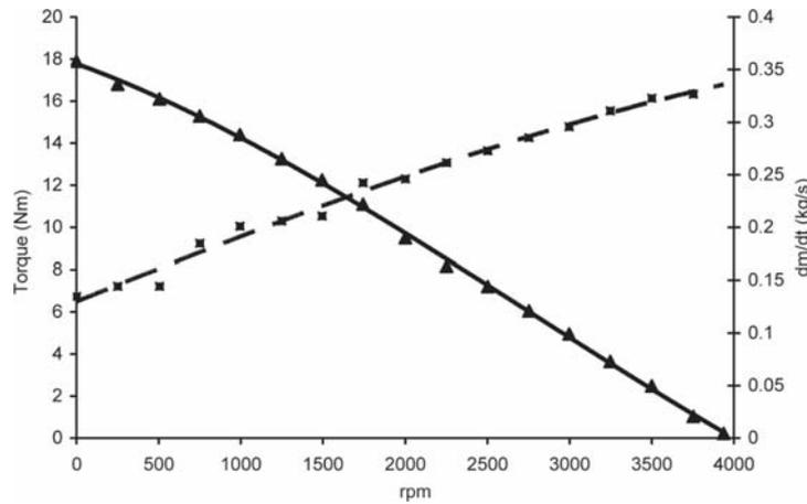
Fig. 6. Variation of torque (continuous line) and mass flow of HFC-134a (dashed line) as a function of the rotation speed.
