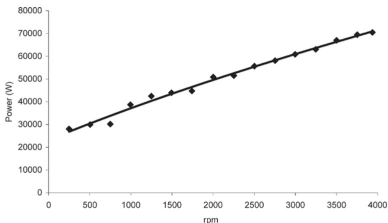
Fig. 9. The overall thermal power generated by the system as a function of the rotation speed.
