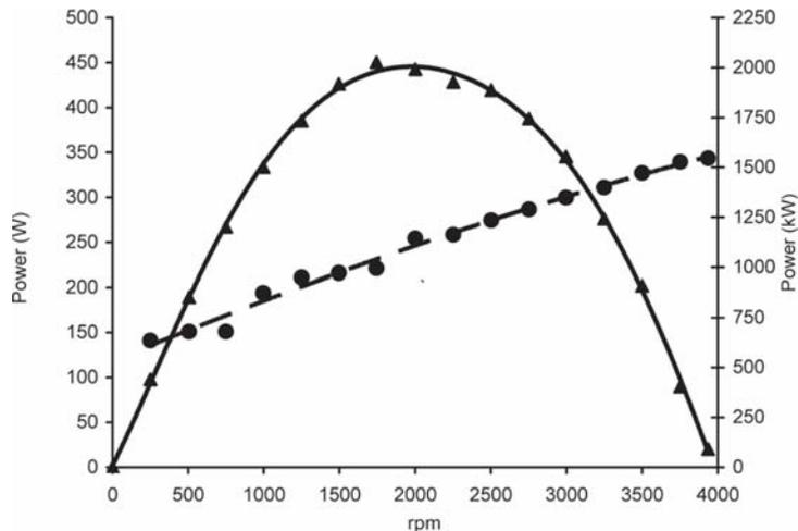
Fig. 7. Variation of power generated by the expander (continuous line, right y axis) and power absorbed by the Freon pump (dashed line, left y axis) as a function of the rotation speed.
